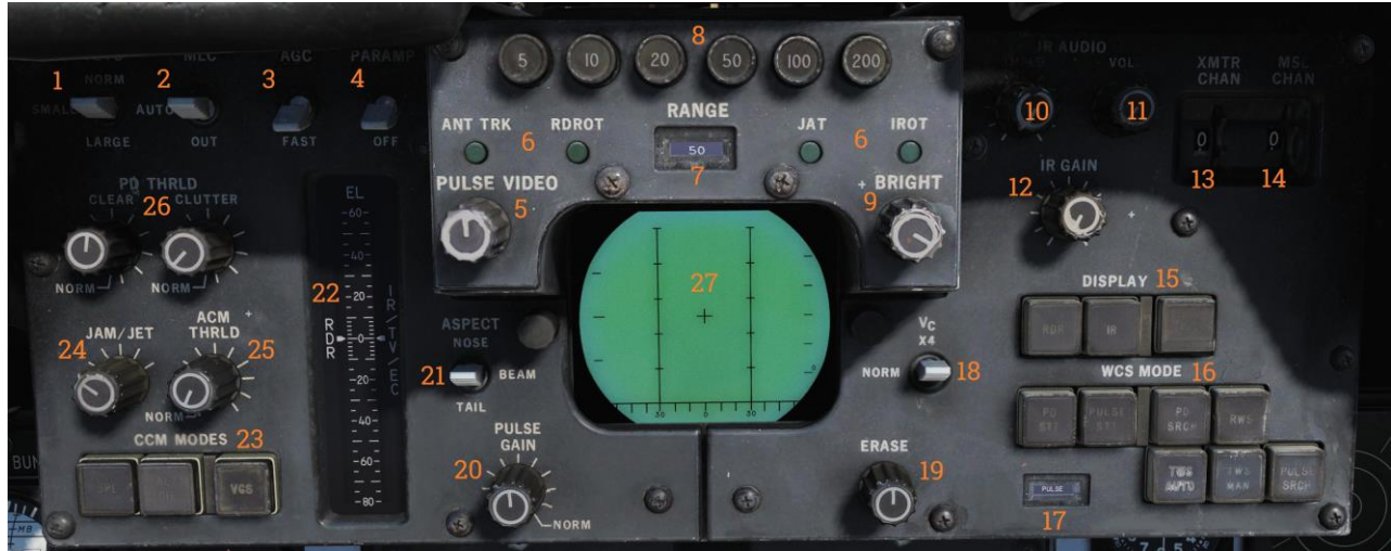
Panel de control principal del radar.
