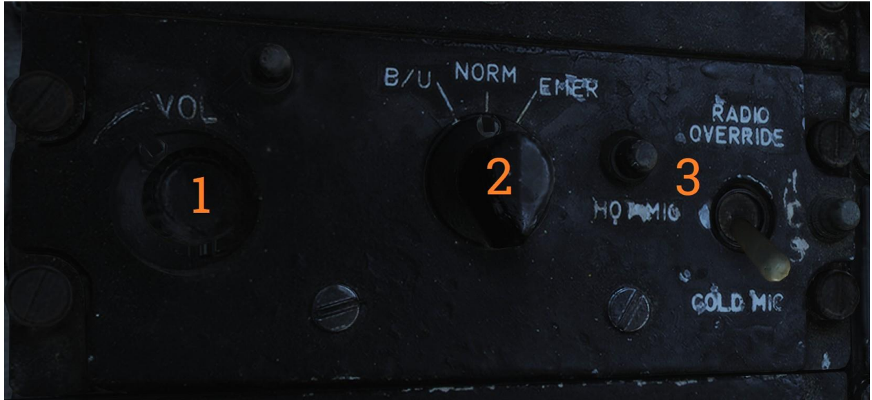
Panel de control del ICS (Intercommunications).
